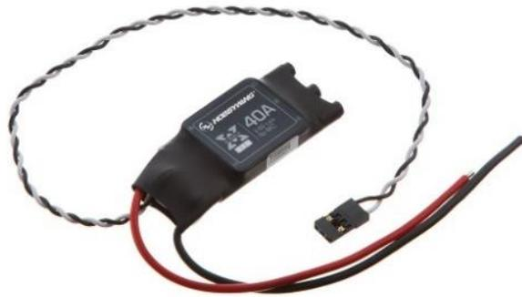
Figura 3.4 Controlador Hobbywing XRotor<sup>11</sup>.
