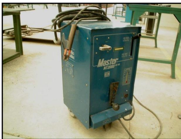
**Figura 3.8 Máquina para soldar (Eutectic Castolin, Master NT2000 AC/DC)**
